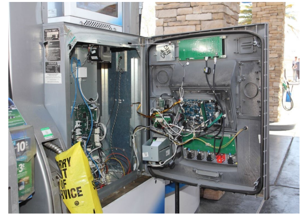
A skimmer behind a gas station pump. Photo courtesy of US Secret Service Las Vegas Field Office
